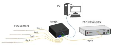
Two of its distinguishing features are the wide range of operating wavelengths from 1250 nm to 1670 nm and the typical switching time of the order of 10 ms. These two features are of particular interest both in optical communication applications, as it operates in the II and III window, and in applications connected to sensors because it allows a fast channel scanning ensuring an optical band compatible with all interrogators operating in the C and L bands used in telecommunications.
